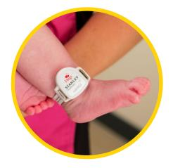
Protection that starts right in the delivery room. As soon as the Hugs tag is attached, the system begins supervising the baby's location and movements. All exits are monitored and a tamper detection feature alerts to unauthorized tag removal. In addition, the solution can be integrated with door security systems to secure the exit against egress.
